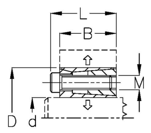
$\begin{array}{lll} \text{B mm} & = 17 \\ \text{d mm} & = 16 \\ \text{D mm} & = 32 \\ \text{Fit tolerance} & = \text{Aksel h8, Nav H8} \\ \text{F kN torque} & = 13 \\ \text{L mm} & = 22 \\ \text{M mm} & = M4 \\ \text{P N/mm2 surface pressure on shaft/hub} = 68 \end{array}$
